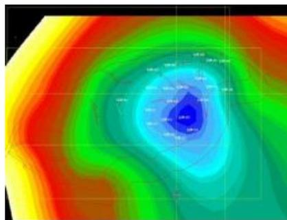
**Figure 9.** Average Velocity Map of Ohaji Oilfield. Colours showing area with the same average velocity
