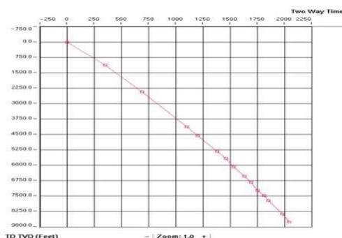
**Figure 2.** Checkshot data T-Z relationship of Ohaji Oilfield
